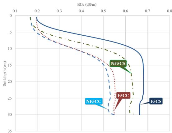
**Fig. 8-** Salt concentration profiles in soil after leaching by MACRO model for continuous treatments with 5 pore volumes of water
