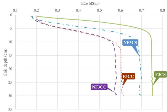
**Fig. 9-** Salt concentration profiles in soil after leaching by MACRO model for continuous treatments with 3 pore volumes of water
