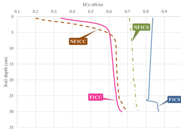
**Fig. 10-** Salt concentration profiles in soil after leaching by MACRO model for continuous treatments with 1 pore volume of water
