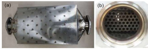
Fig. 10. Photos of (a) exhaust HEX, (b) perforated plate placed inside [20].
