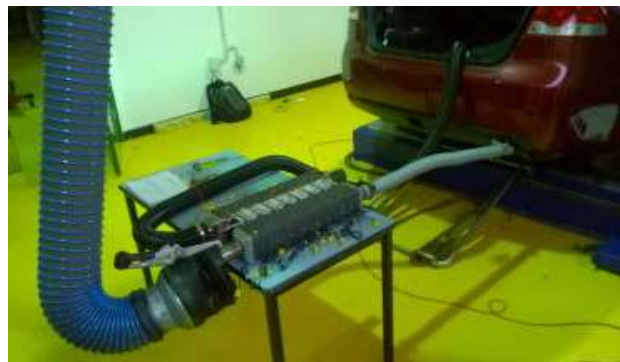
Fig. 74. TEGs/heat pipes system inside lab, reprint with permission.
