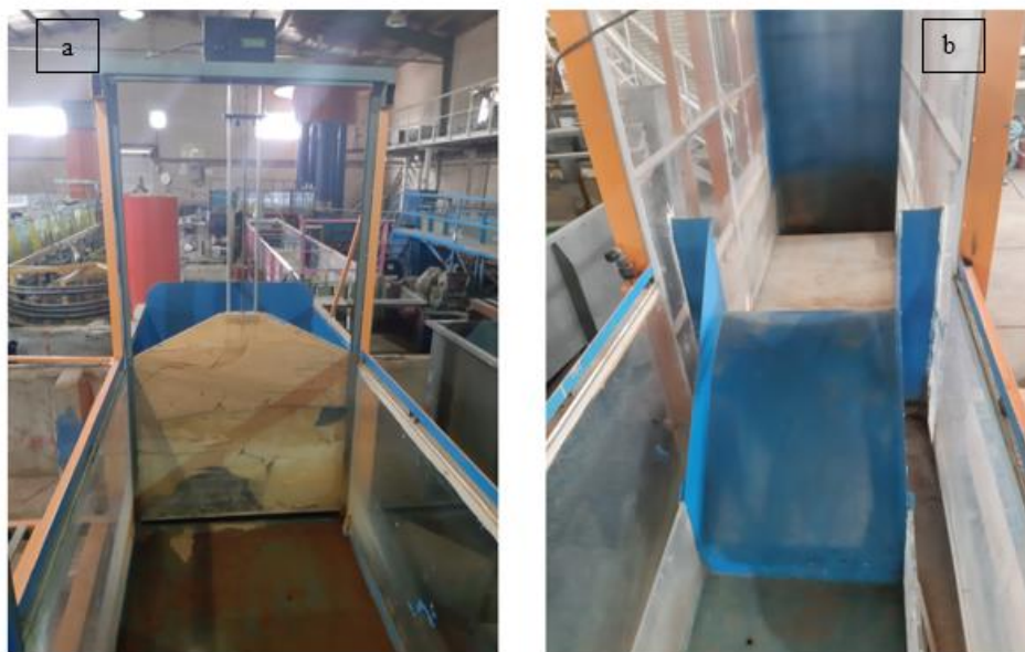
Figure 3- A view of the gate of the flume (a) and the ogee spillway (b)
