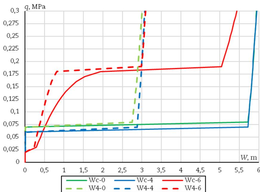
Fig. 4. Graph of deflection versus load for different number of weakening for shell option 1.
