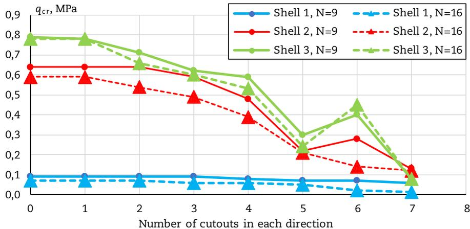
**Fig. 3.** Critical load values for different number of attenuations.
