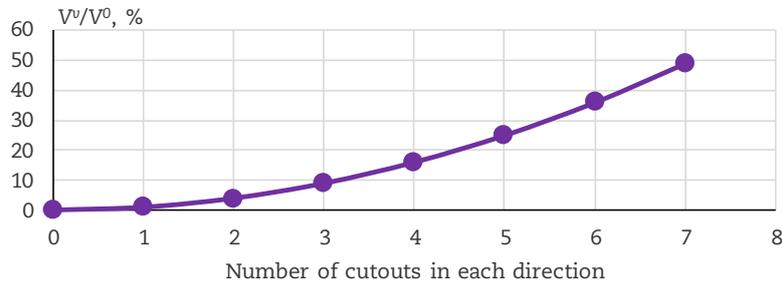
**Fig. 2.** The ratio of the volume of cutouts to the volume of shell skins depending on the number of cutouts in each direction.
