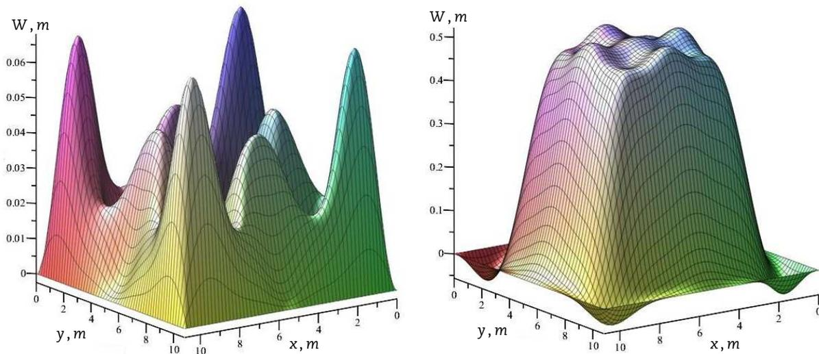
Fig. 6. Deflection fields of the shell option 3 with the number of cutouts  $6 \times 6$ .
