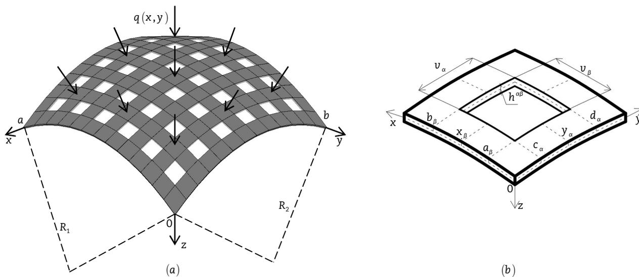
Fig. 1. Shallow shell with double curvature: (a) Design scheme; (b) Cutout geometry.
