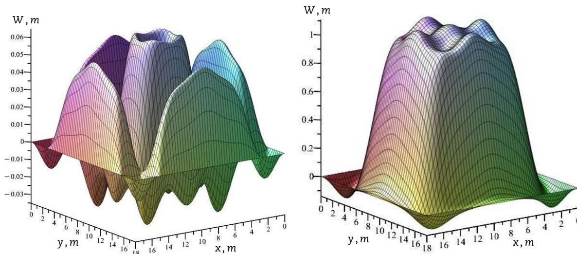
Fig. 5. Deflection fields of the shell option 2 with the number of cutouts  $6 \times 6$ .
