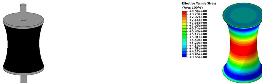
(a) The AE42 specimen: the black colour is for rubber and the silver colour is for metal.
