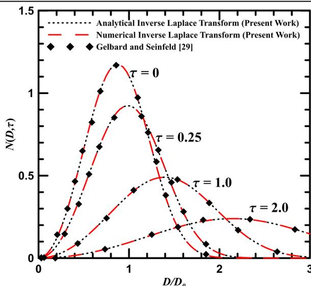
Fig. 5. Comparison of  $N(D, \tau)$  distribution for both coagulation and particle growth with constant kernel (test-case 3).
