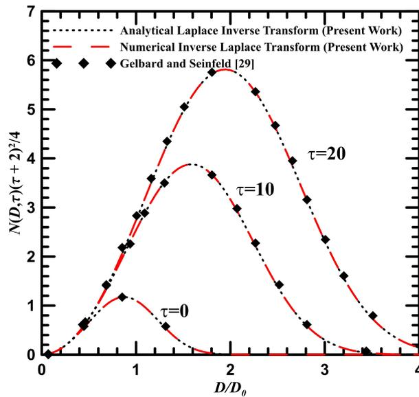
Fig. 3. Comparison of  $N(D, \tau)$  distribution for pure coagulation with constant kernel and ratio  $(D/D_0)$  in the range  $[0,4]$  (test-case 1).
