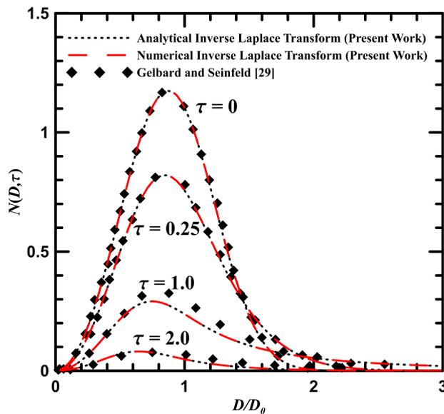
Fig. 4. Comparison of  $N(D, \tau)$  distribution for pure coagulation with varying kernel (test-case 2).
