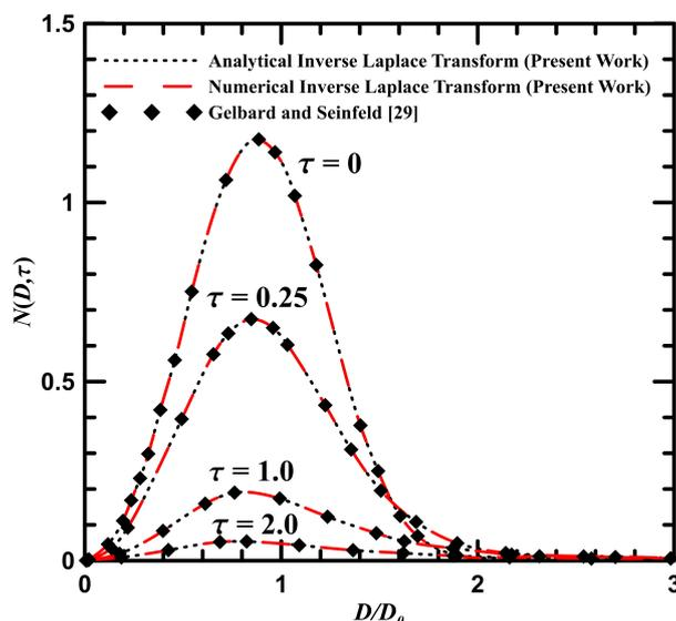
Fig. 6. Comparison of  $N(D, \tau)$  distribution for coagulation with varying kernel and removal rate (test-case 4).
