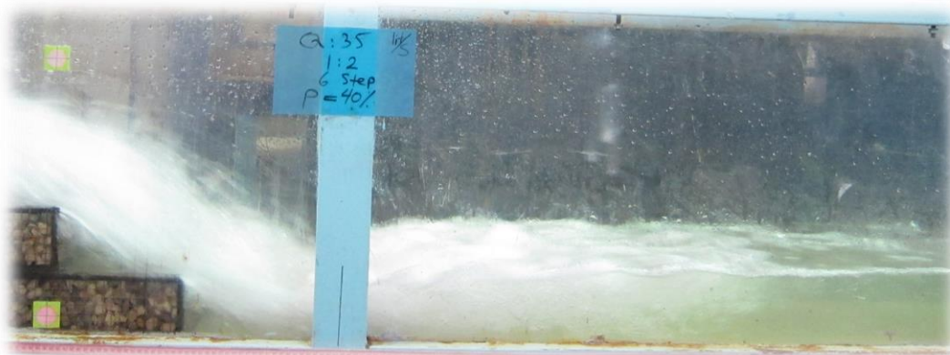
Fig. 4- Creation of hydraulic jump downstream of gabion stepped spillway with 40% porosity at 35 (l/s) discharge
