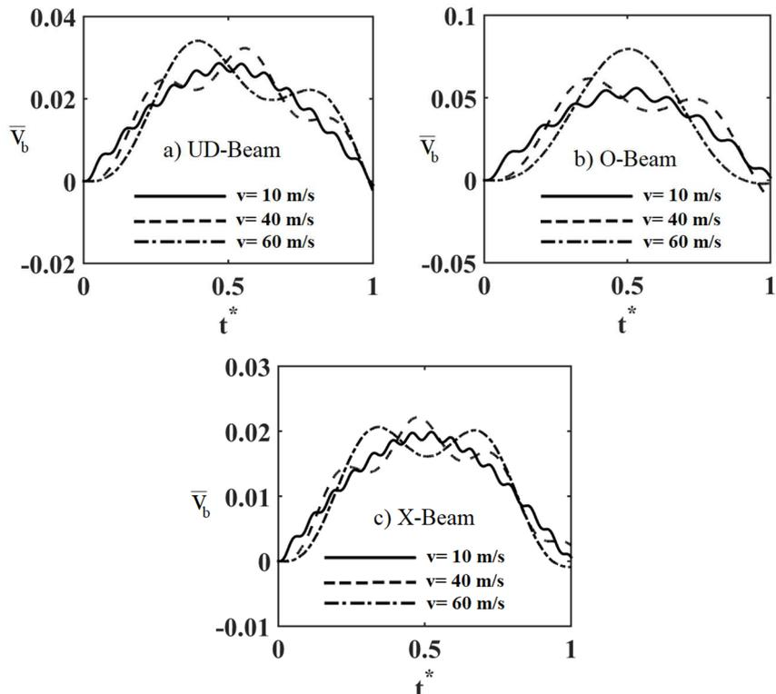
Fig. 4. Time history of dimensionless dynamic displacements at midspan of CNTRC beam with different reinforcement patterns and the velocities of load for volume fraction of CNTs  $V_{CNT}=0.17$ .
