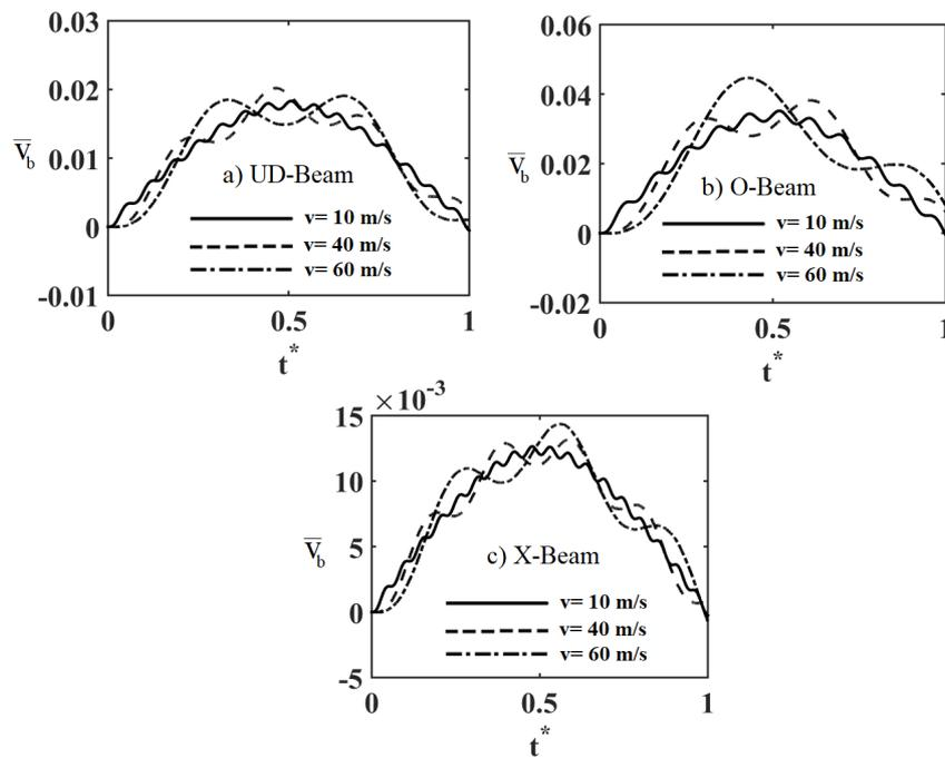
Fig. 5. Time history of dimensionless dynamic displacements at midspan of CNTRC beam with different reinforcement patterns and the velocities of load for volume fraction of CNTs  $V_{CNT}=0.28$ .
