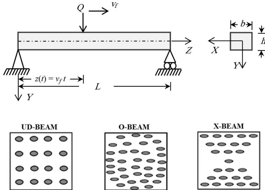
Fig. 1. A schematic configuration of a simply supported CNTRC beam under a moving load and three different patterns of CNTs.
