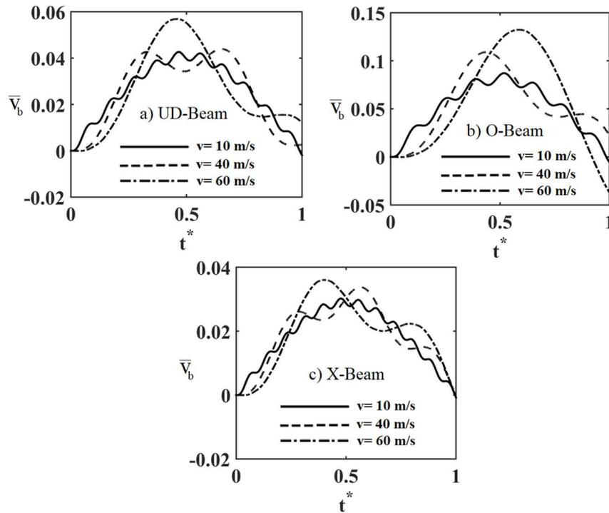
Fig. 3. Time history of dimensionless dynamic displacements at midspan of CNTRC beam with different reinforcement patterns and the velocities of load for volume fraction of CNTs  $V_{CNT}=0.12$ .
