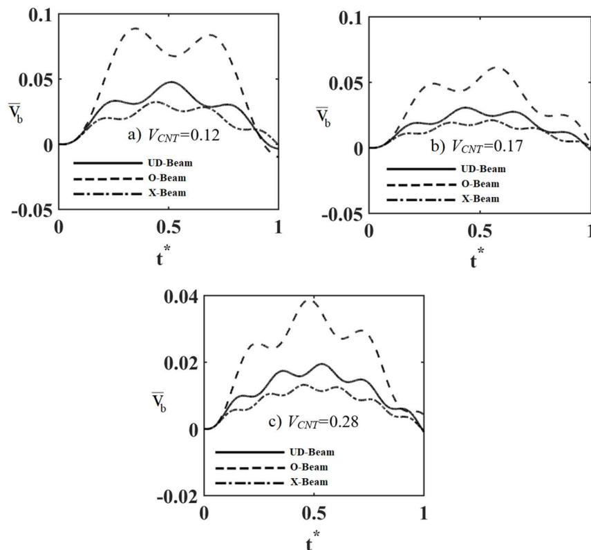
Fig. 2. Time history of dimensionless dynamic displacements at midspan of CNTRC beam with different reinforcement patterns and volume fraction of CNTs.
