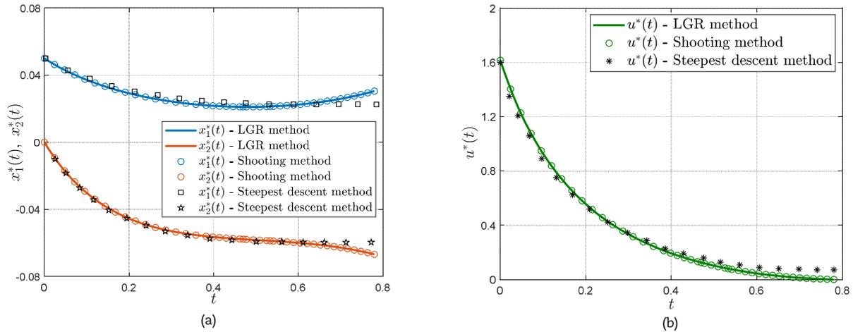
Fig. 5. (a) Optimal states and (b) the optimal control for the continuous stirred-tank chemical reactor with LGR (solid lines) and with the shooting and steepest descent (scattered points) methods.
