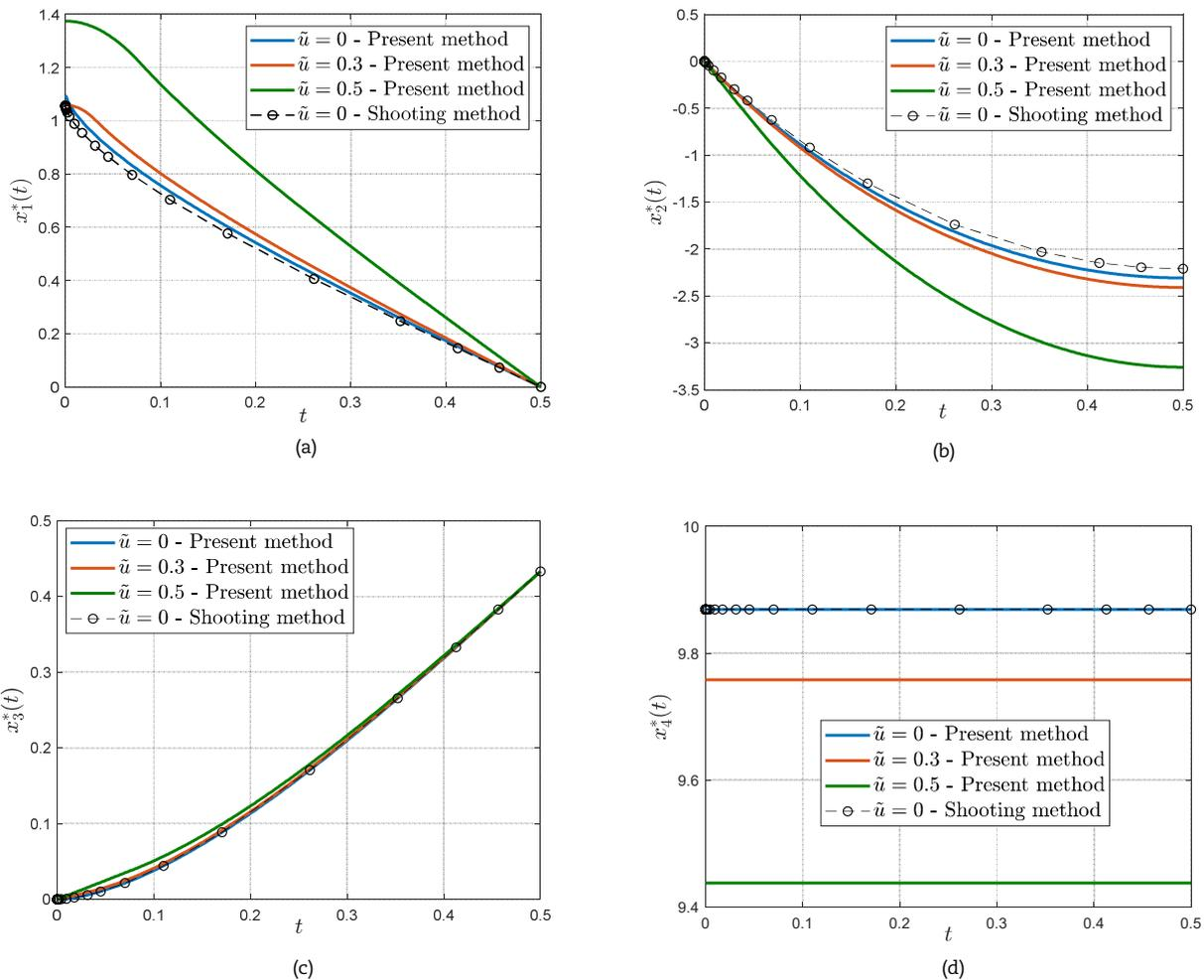
Fig. 3. Optimal states for Lagrange's column with different constraints on the minimal value of the control function  $\tilde{u}$ .
