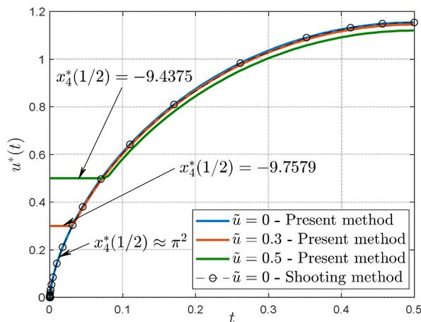
Fig. 4. Optimal cross-sectional area distributions for Lagrange's column with different constraints on the minimal value of the control function  $\tilde{u}$ .
