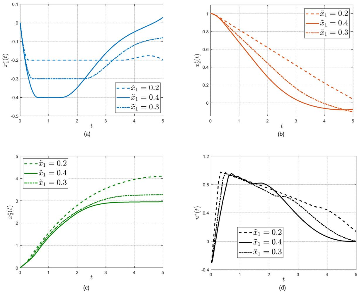
Fig. 6. (a, b, c) Optimal states and (d) input function for the Van der Pol oscillator problem with three constraints on the minimal value of the state  $x_1$ .
