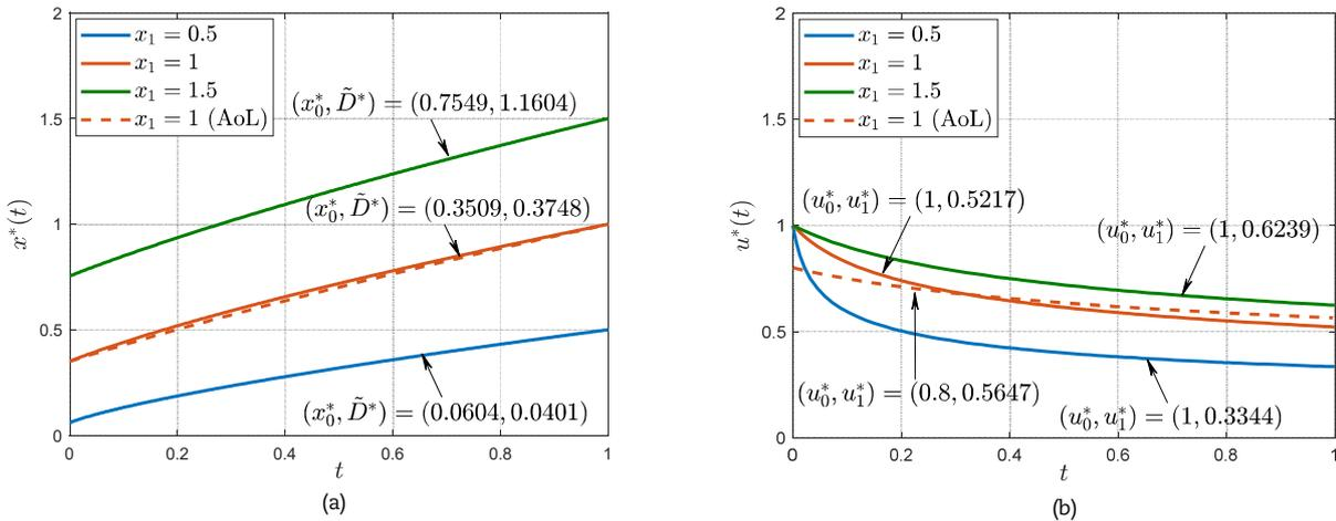
Fig. 2. (a) Optimal meridian profiles for Newton's body with different values of  $x_1$  by means of the LGR method (solid lines) and the analytical closed-form solution in eq. (32) with  $x_1 = 1$  (dashed line). (b) Optimal input functions with illustration of the Weierstrass-Erdmann condition at  $t = 0$ .
