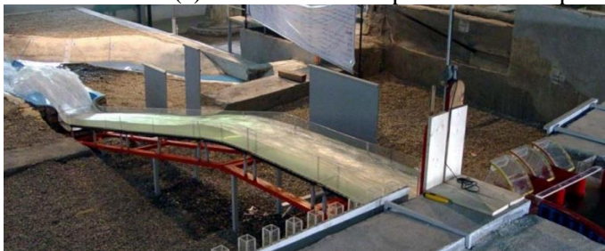
(b) The physical model at a scale of 1:50
