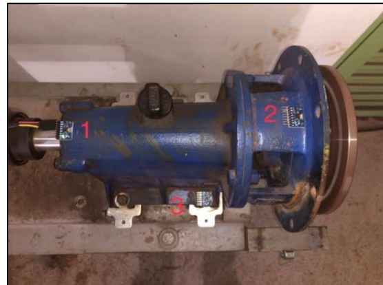
Fig. 7. Positioning of Vibration Sensors
