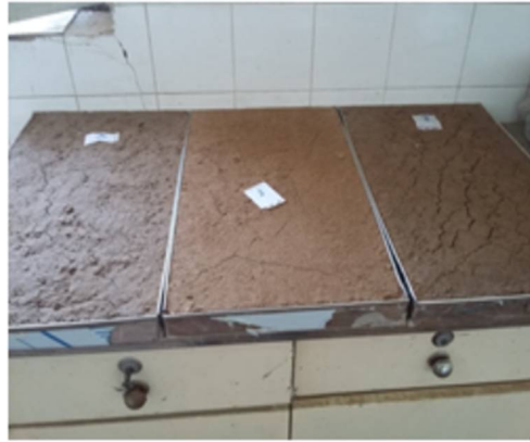
Fig. 3: Pseudo undisturbed and wetted soil sample
