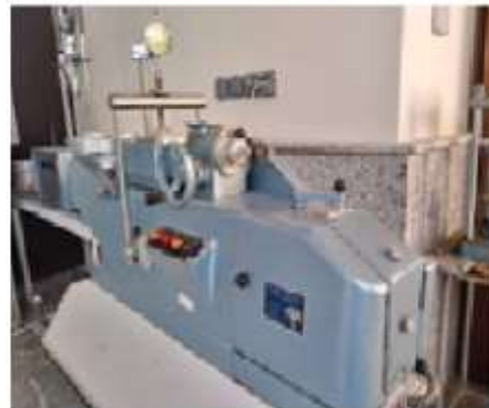
Fig. 4- Direct shear test equipment (a) direct shear (b) sample in the straight cut
