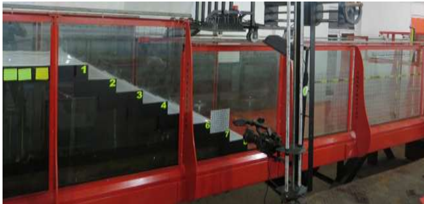
Fig. 1- Flume, Spillway, LED, Rail, and Location of Camera (Slope 1:2, \theta=27.5^\circ )
