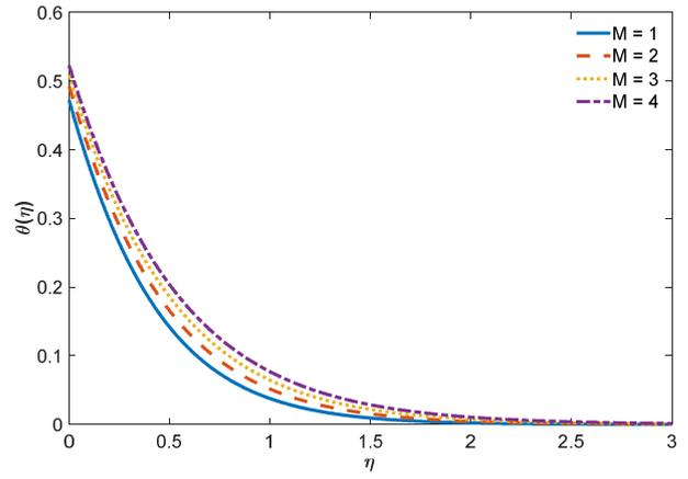
Fig. 9. Temperature description for diverse magnetic variable  $M$
