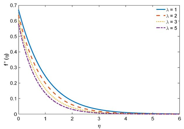
Fig. 5. Velocity field for diverse slip velocity parameter  $\lambda$
