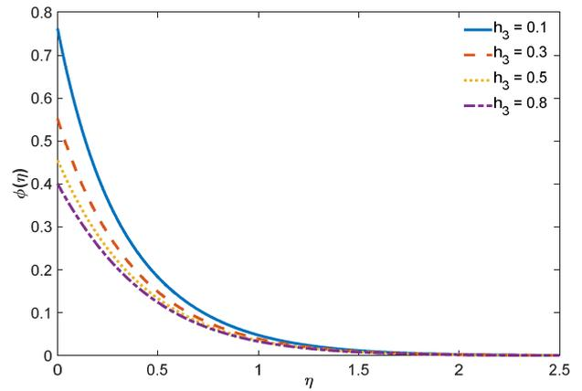
Fig. 33. Mass profile for diverse values of concentration slip variable  $h_3$
