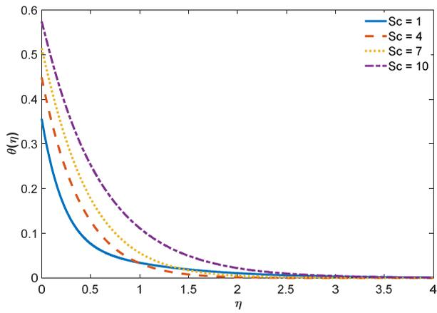
Fig. 14. Temperature field for diverse Schmidt number  $Sc$
