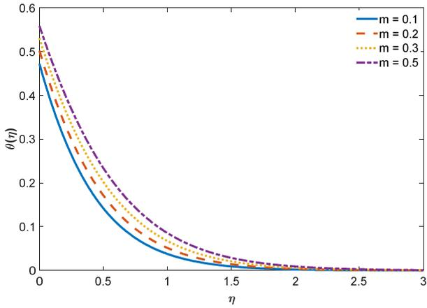
Fig. 8. Temperature field for diverse values of  $m$
