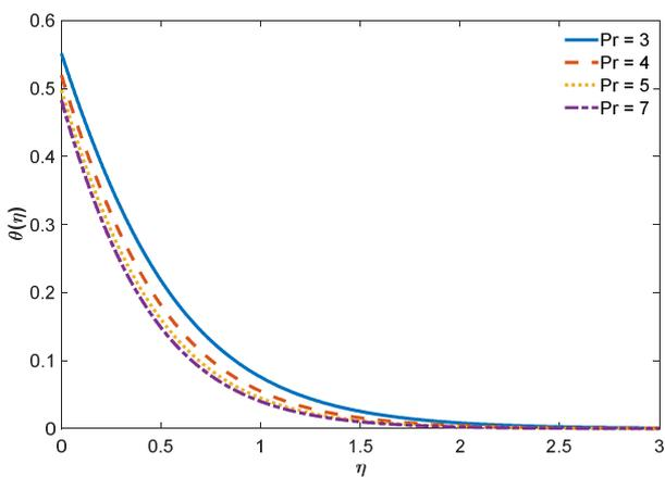
Fig. 12. Energy field for diverse Prandtl number  $Pr$
