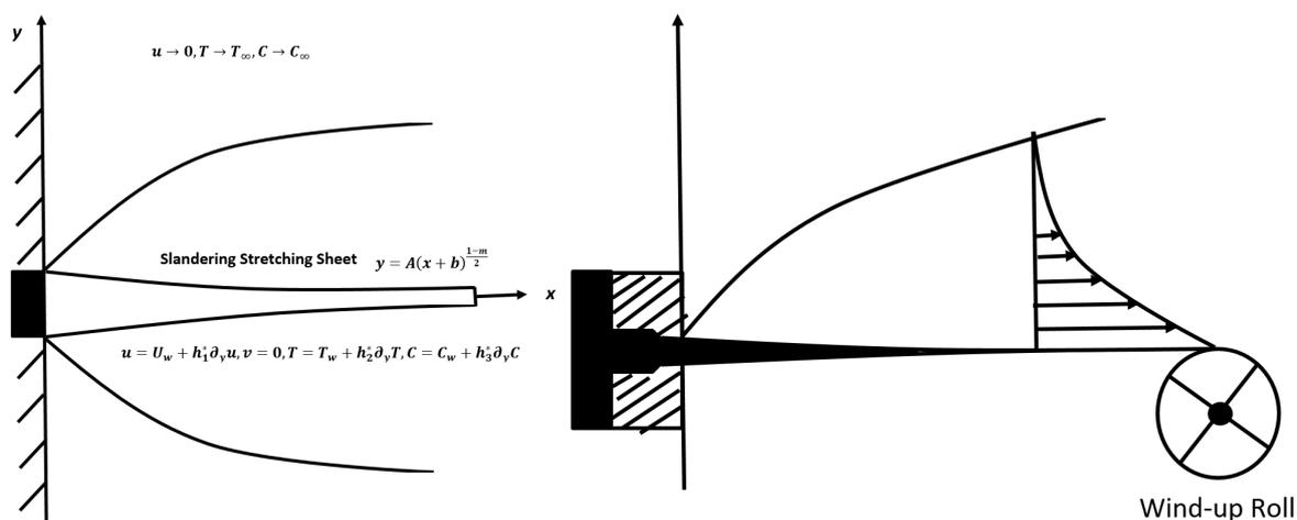
Fig. 1. Schematic diagram of the problem with engineering application in wind-up roll
