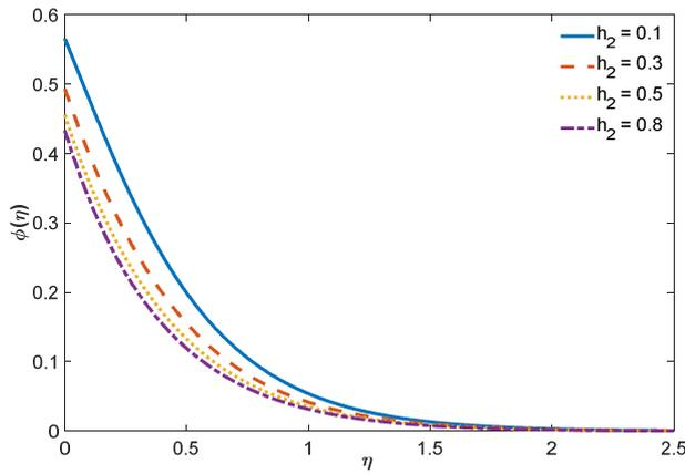
Fig. 32. Mass field for diverse values of temperature slip variable  $h_2$
