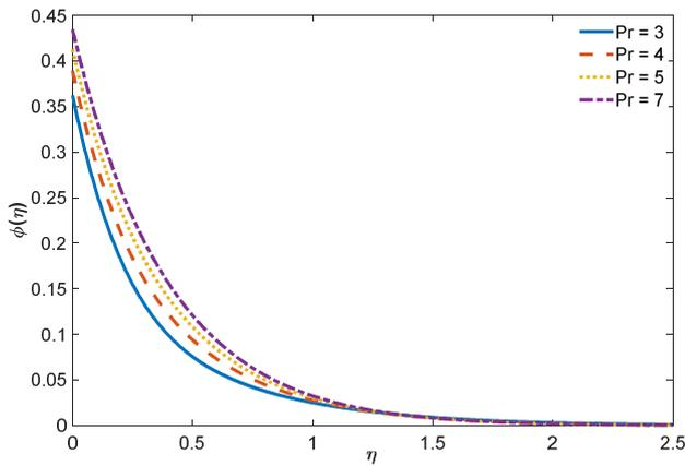
Fig. 26. Mass profile for diverse values of Prandtl number Pr
