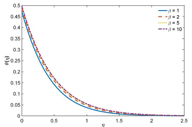
Fig. 7. Temperature field for diverse Casson variable  $\beta$
