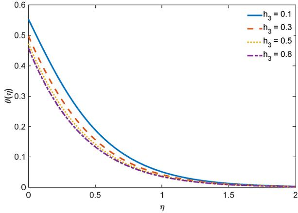
**Fig. 20.** Temperature profile for diverse values of concentration slip parameter  $h_3$
