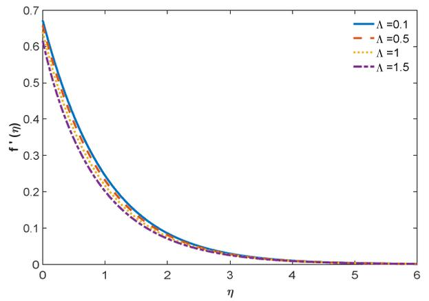
Fig. 3. Velocity field for diverse Williamson parameter  $\Lambda$
