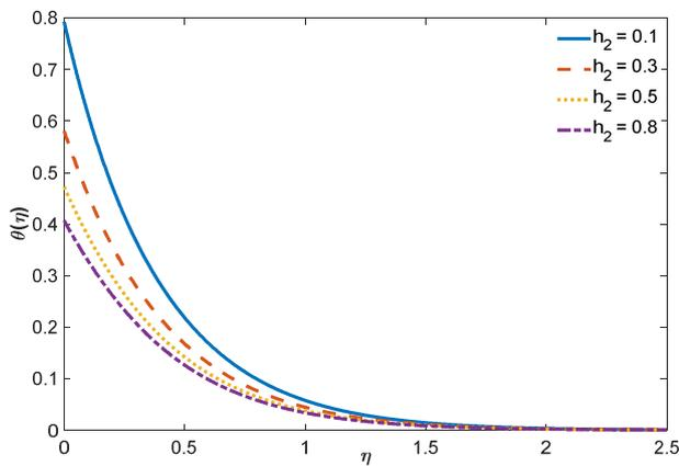
Fig. 18. Energy description for diverse values of temperature slip var.  $h_2$
