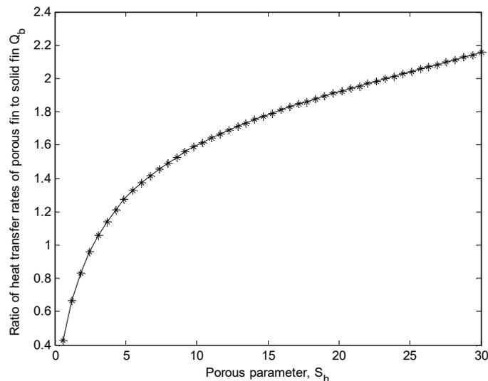
Fig. 10. Thermal performance ratio of the porous fin
