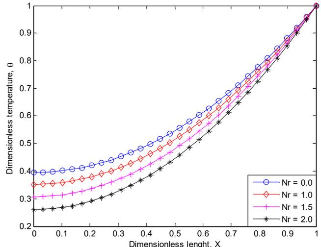
Fig. 7. Effects of radiative parameter on the nondimensional temperature distribution in the fin
