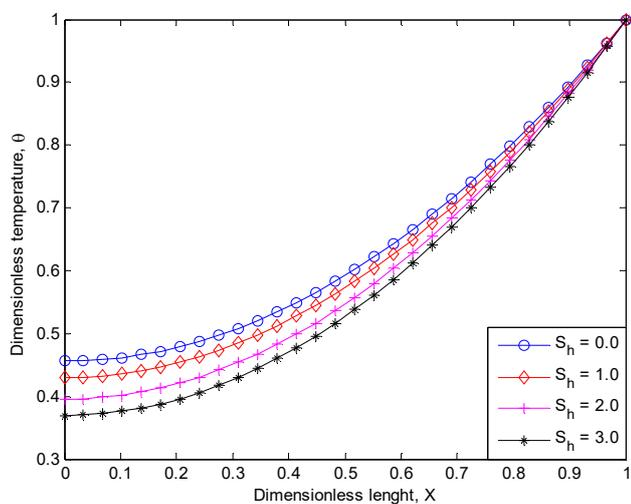
Fig. 8. Effects of porous parameter on the nondimensional temperature distribution in the fin
