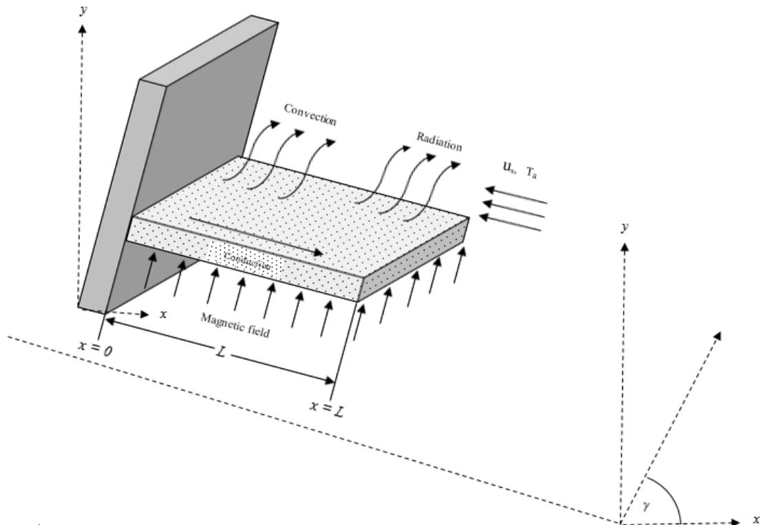
Fig. 2. Schematic configuration of convective-radiative longitudinal porous fin inclined at an angle  $\gamma$  to the horizontal axis
