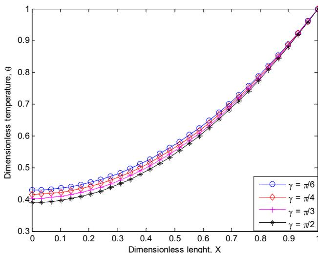
Fig. 4. Effects of inclination of fin on the nondimensional temperature distribution in the fin
