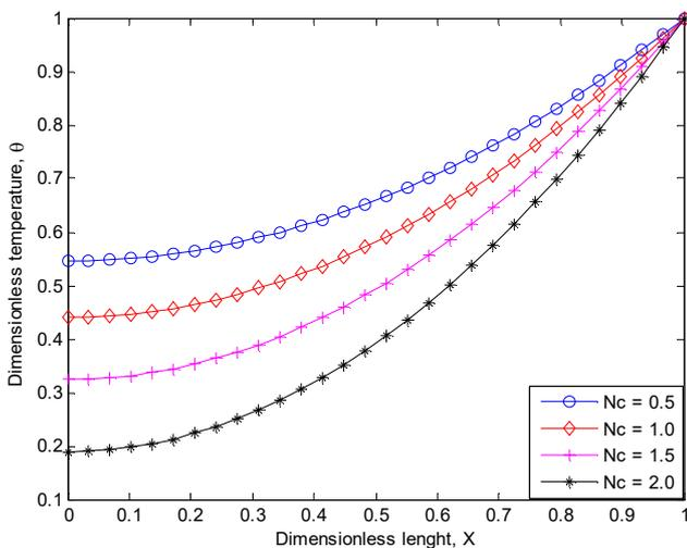
Fig. 6. Effects of convective parameter on the nondimensional temperature distribution in the fin
