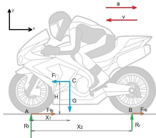
Fig. 2. The system of forces acting on the braking motorcycle.
