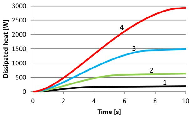
Fig. 5. Heat dissipated to atmosphere through radiation and convection: 1- initial speed 100 km/h, 2- initial speed 150 km/h, 3- initial speed 200 km/h, 4- initial speed 250 km/h.
