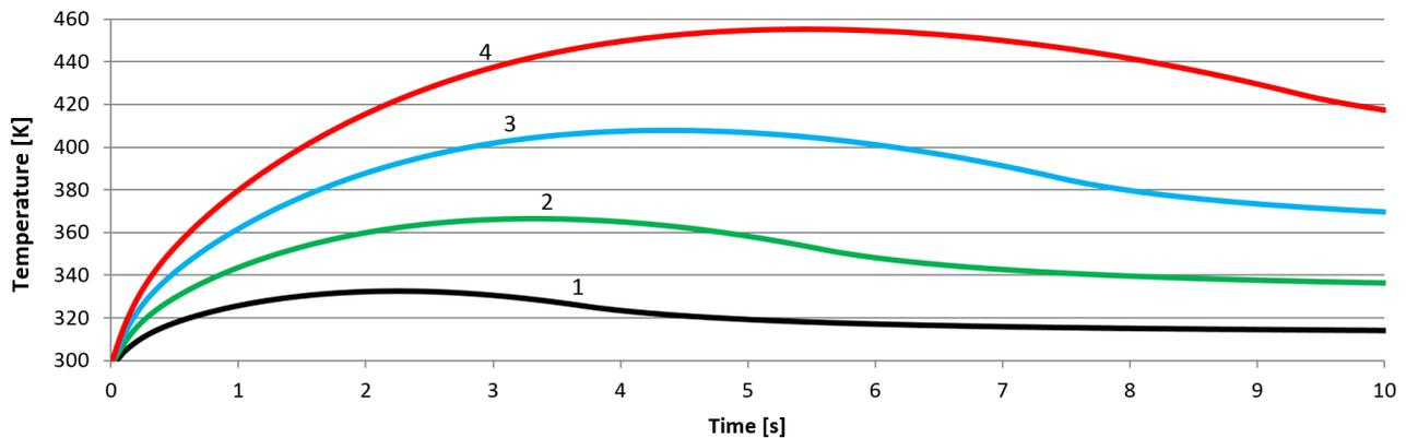
Fig. 4. Course of heating process of brake disc :1- initial speed 100 km/h, 2- initial speed 150 km/h, 3- initial speed 200 km/h, 4- initial speed 250 km/h.
