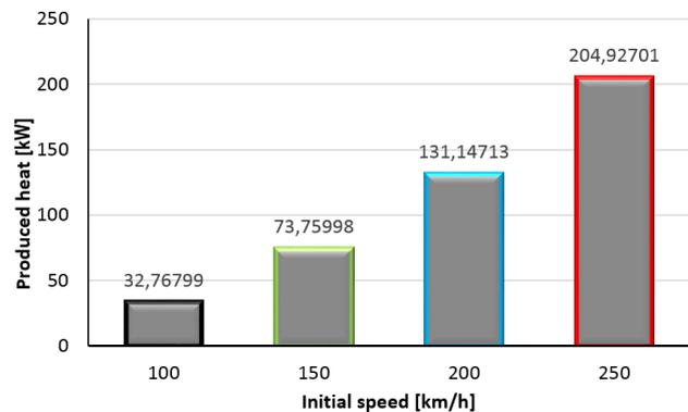
Fig. 6. Amount of heat produced in braking process
