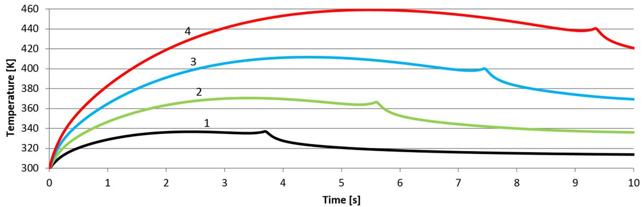
Fig. 3. Course of heating process of brake pad :1- initial speed 100 km/h, 2- initial speed 150 km/h, 3- initial speed 200 km/h, 4- initial speed 250 km/h.
