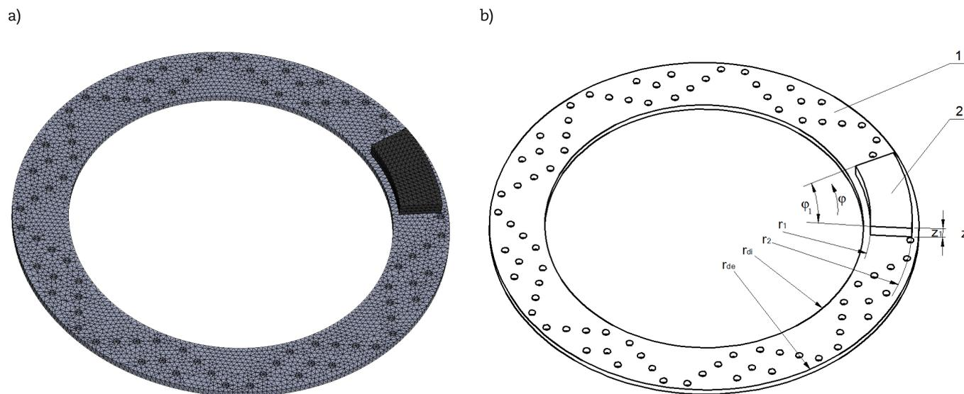
**Fig. 1.** CAD model of object of research: a)covered by mesh, b)with geometry markings.
