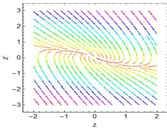
**Fig. 1.** Depicts the phase portrait for a stable node in a system having the particulars:  $P = 0.5, \mu = 0.0, \eta = 1.0, \omega = 1.0$  and  $Q = 1.0$
