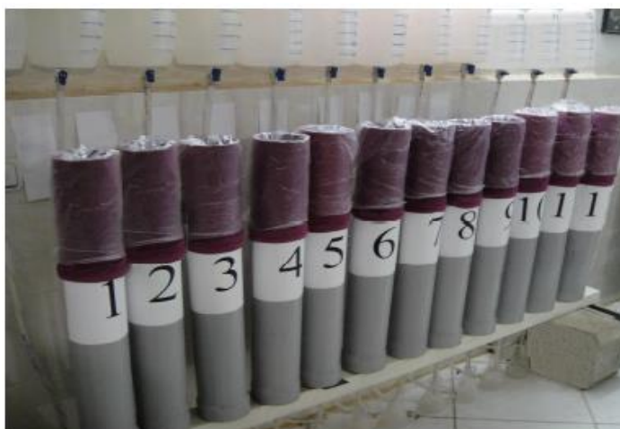
Fig. 2-Physical Designed model for desalinization and desodification
