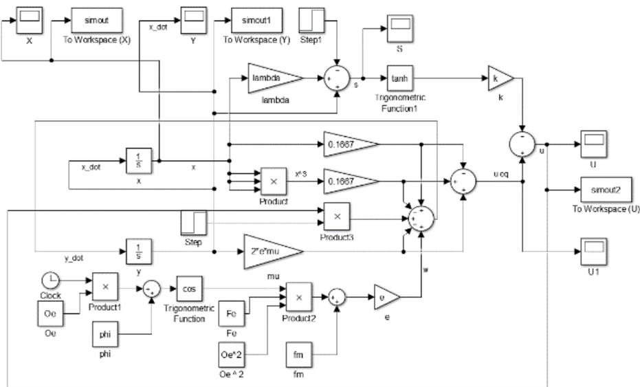
Fig. 14. Gear transmission system and sliding mode controller in MATLAB Simulink
