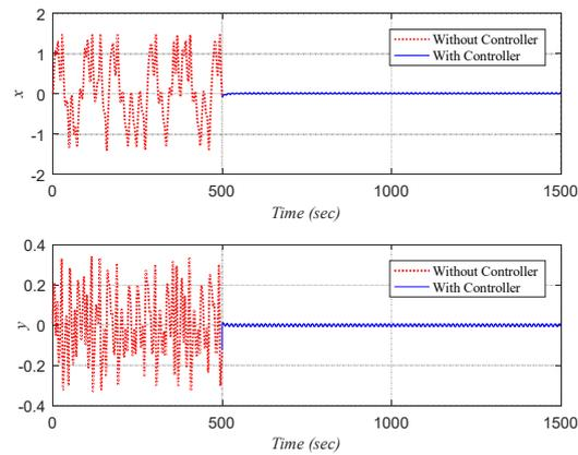
Fig. 16. Time history of state space variables with  $f_e = 30$ , after applying SMC control input
