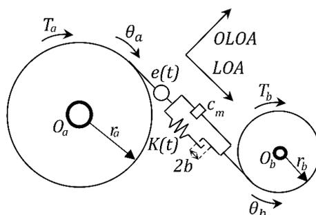
Fig. 1. Gear transmission system dynamic model [18]
