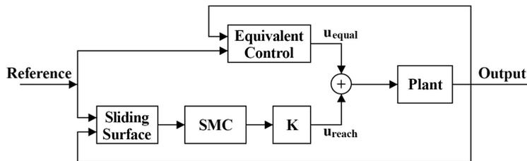
Fig. 13. SMC Controller Structure
