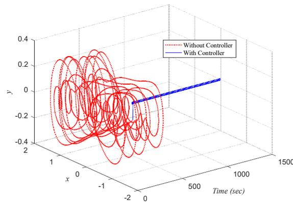
Fig. 17. 3D Phase plane with  $f_e = 30$ , after applying SMC control input
