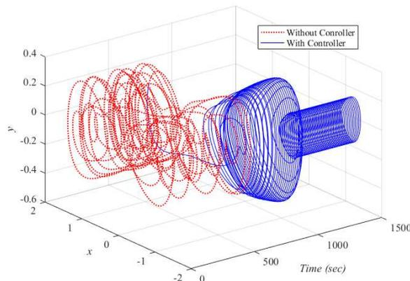
Fig. 12. 3D Phase plane with  $f_e = 30$  , after applying GPC control input
