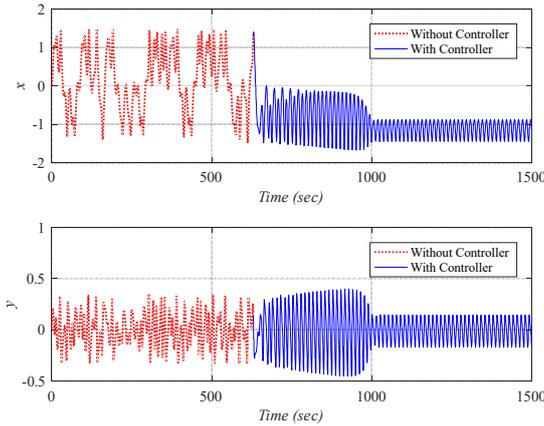
Fig. 10. Time history of state space variables with  $f_e = 30$  , after applying GPC control input
