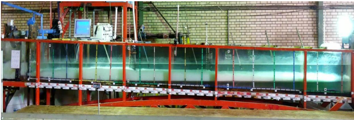
Fig.1- Motion of the interflow density current in a horizontal layer whit saline stratification
