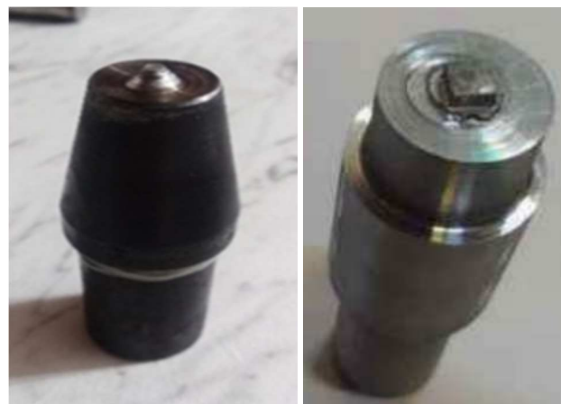
Fig. 3. Hot steel welding cylindrical tool with square and cylindrical pin
