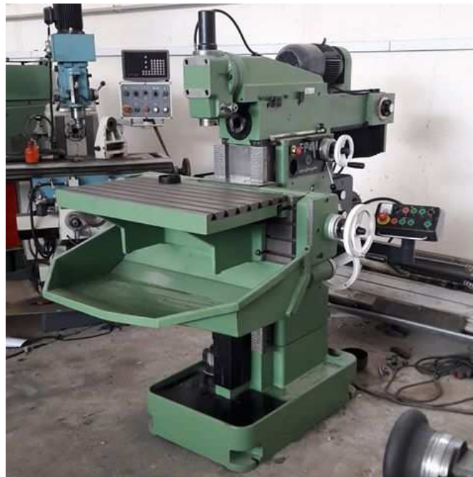
Fig. 2. FP4M milling machine used in experimental tests
