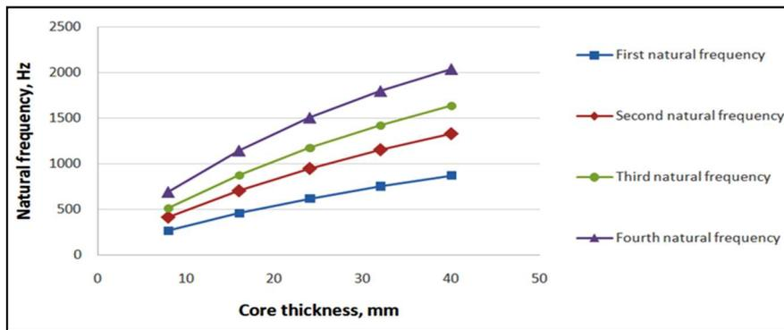
Fig. 10. Influence of core thickness on natural frequency
