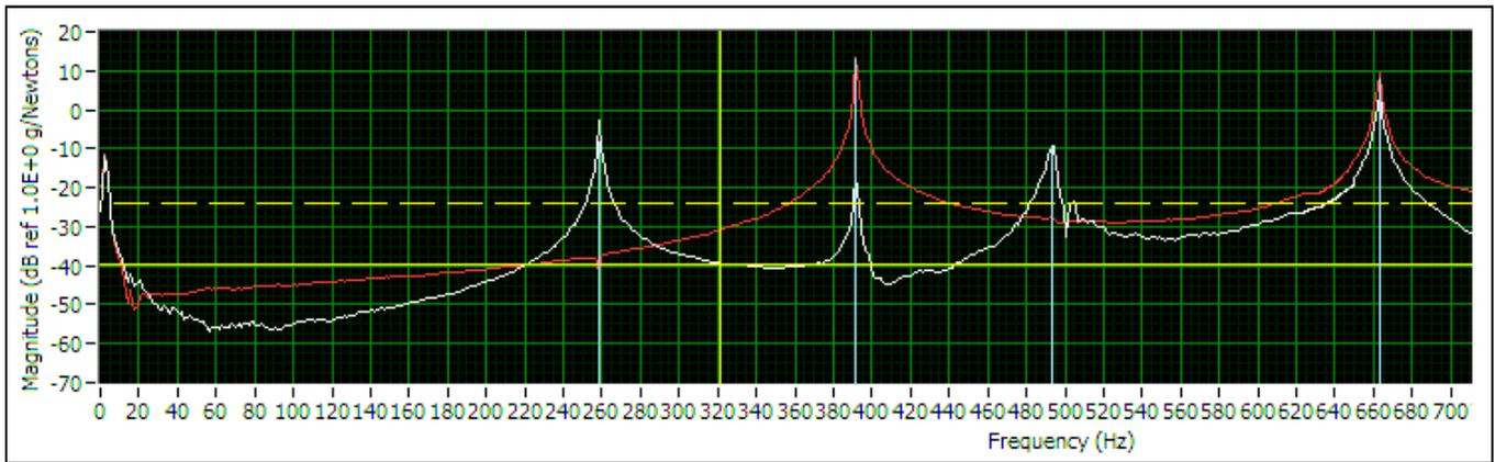
Fig. 8. Experimental modal testing results
