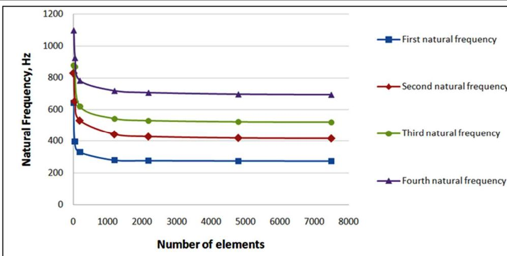
Fig. 2. Mesh sensitivity analysis of plate modal analysis (SVS)
