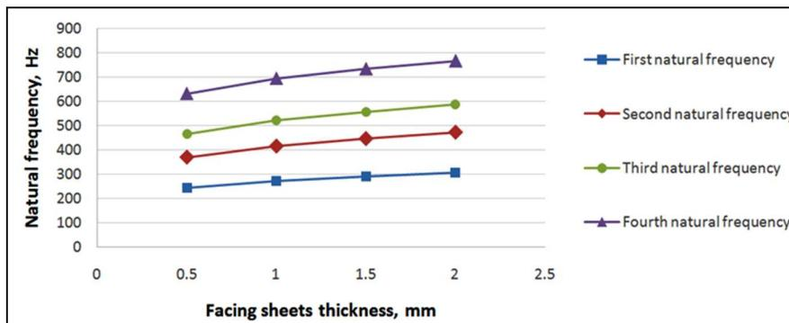
Fig. 11. Influence of facing sheets thickness on the natural frequency
