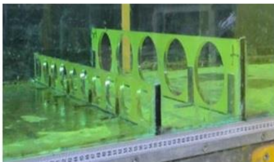
Fig.4- View of perforated sills. A) Schematic of perforated sills. B) View of the plexiglass perforated sills in the experiments
