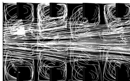
Fig. 18- he top view of flow pattern in the Daniel fishway with a baffle angle of 45 °
