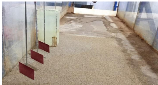
Fig. 3- Photograph of the Flume, abutment and immersed vanes
