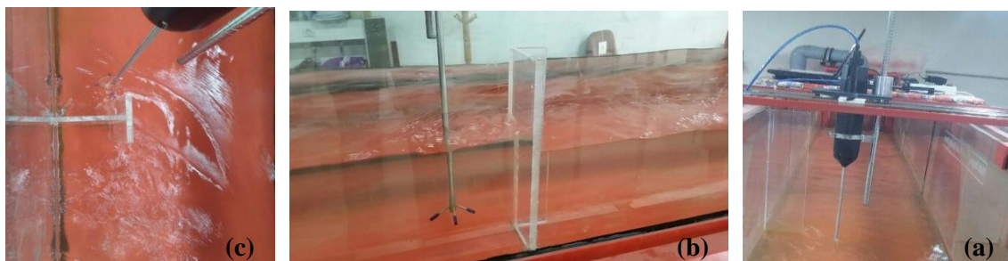
Fig. 4- ADV device during measuring of flow velocity (a) Straight groyne (b) L-shape groyne and (c) T-shape groyne
