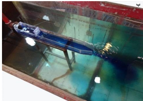
Fig. 1- Convergent surface jet in an experimental run
